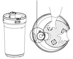
**IMPORTANT:** IN ROUND BRINE TANK, IT IS IMPORTANT TO ALIGN THE HANDLE TO THE BRINE WELL AS SHOWN.
