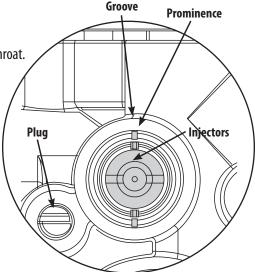
PLEASE NOTE: Make sure the two prominences on the injector are aligned to the grooves on the valve body.
