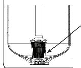
The riser (distributor) remains inside the tank seated in the depression at the bottom
