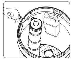
**4.** IInstall the holder and the Res Care Solution **5.** Take off the small hole cover on the Brine Well lid.
