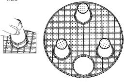
**2.** Insert the brine well assembly inside and below the grid plate.
