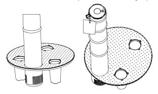
**3.** Place the brine grid with the brine well inside the brine tank such that the nut fitting faces the hole on the brine tank. Then press the grid evenly inside the brine tank until the brine grid legs and the brine well, as an assembly, touch the bottom of the brine tank.
