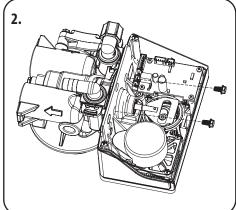
**2.** Remove two (2) bolts securing powerhead to **3.** Remove powerhead from body.
