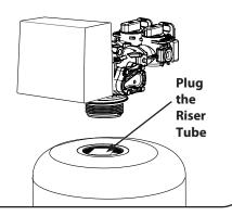
**2.** Ensure the bottom of the riser tube remains seated in the depression at the bottom of the tank. Fill tank one-quarter full with water to protect the distribution tube during gravel installation.
