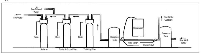
NOTE: A neutralizing filter is the first unit installed in a water system after the outdoor raw water lines (\*) when pH correction is required.
